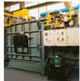
Air/gas ratio control on melting furnace for ensuring stoichiometric combustion over the entire capacity range
